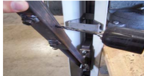
Figure 8.3b. Drilling out the Arms
