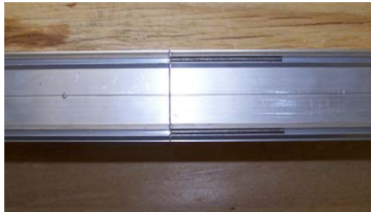
Figure C.6.c. Installing Chain Guide Sections
