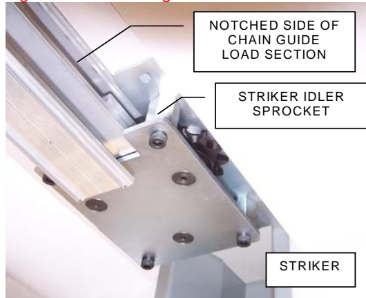
Figure C.4.b. Installing Striker Load Section.
