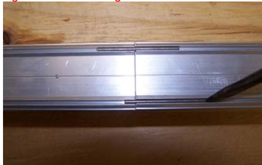
Figure C.6.d. Positioning Alignment Pins
